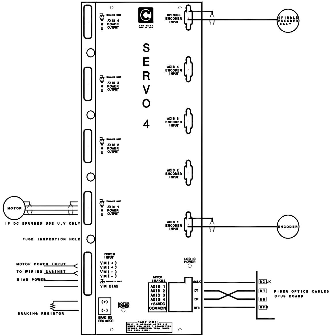
Motor power and encoder cables should not be run together. Only specified connectors are to be used.
