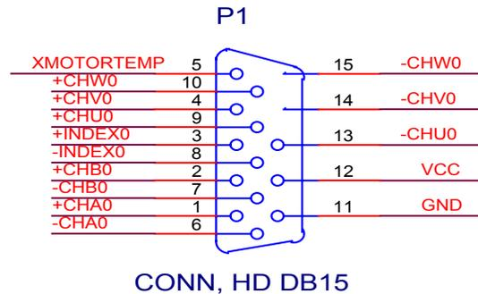
**Spindle Encoder Input** This input does not require commutation channel and is compatible to previous wiring.
