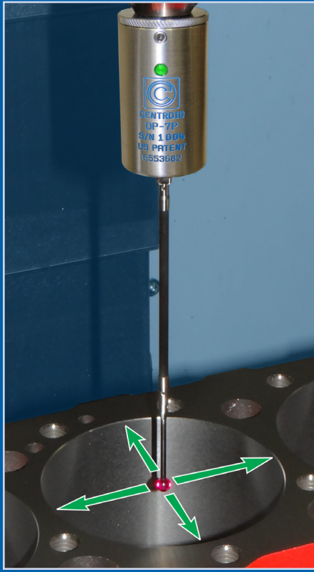
Automatic Part Setup with CNC Probing Cycles*
