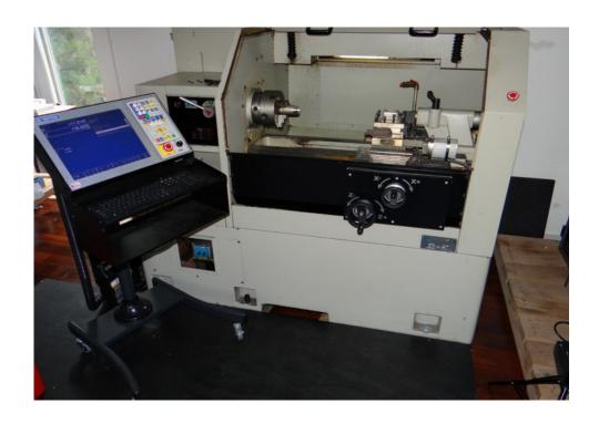
Horizontal flat bed structure, hardened box guide way with high temperature quenching
