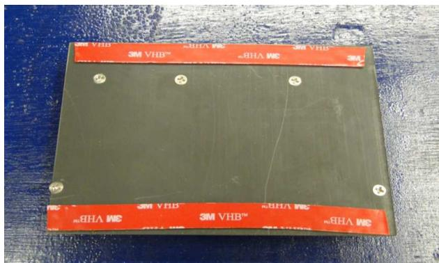
5. Install the OpticDirect unit on to the Delta Drive on the right side flush with the front and the ribbon cable lined up with the CN1 connector, not exceeding flush with the top. Making sure the tape is well seated. A 750 watt drive is shown.
