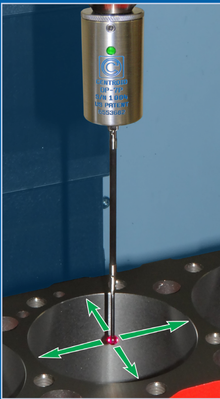
Automatic Part Setup with CNC Probing Cycles*
