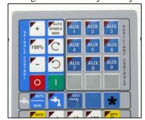
\*The M13/M14 commands require that the AUX12 jog panel key be pressed. The AUX12 key must be held down continually until the carousel and clamp switches are in the default state or a stop condition will result. The AUX12 key is the unlabeled blue key located in the rightmost column of the coolant section (right of the mist key and below the tool index + key). AUX12 is indicated by the \* in the picture to the left.
