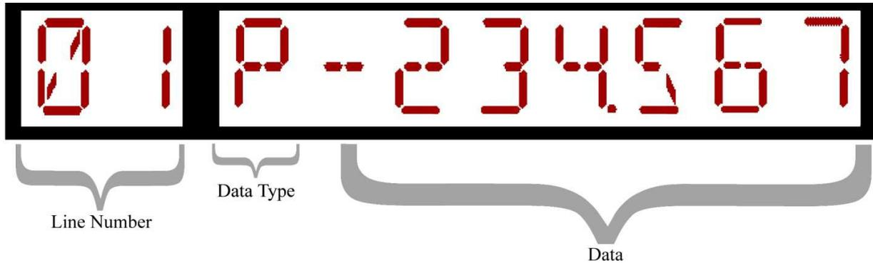
**Line Number** - In run mode, this is the line number that is executing. In program mode, this is the line that is being displayed or edited. In config mode, this is the parameter number that is being displayed or edited.
