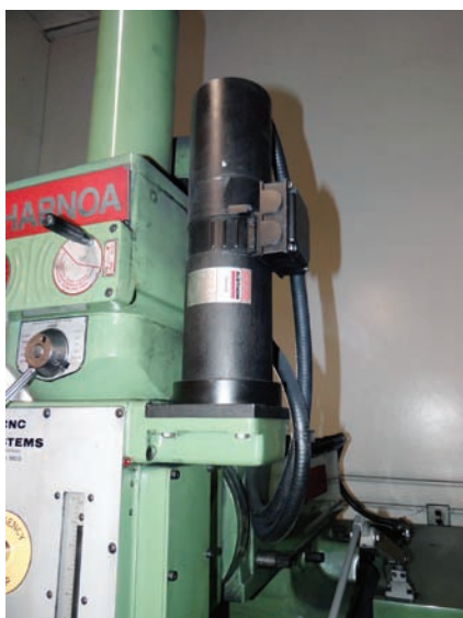
The original servo motors were retained during the Sharnoa's upgrade (Z-axis shown).
