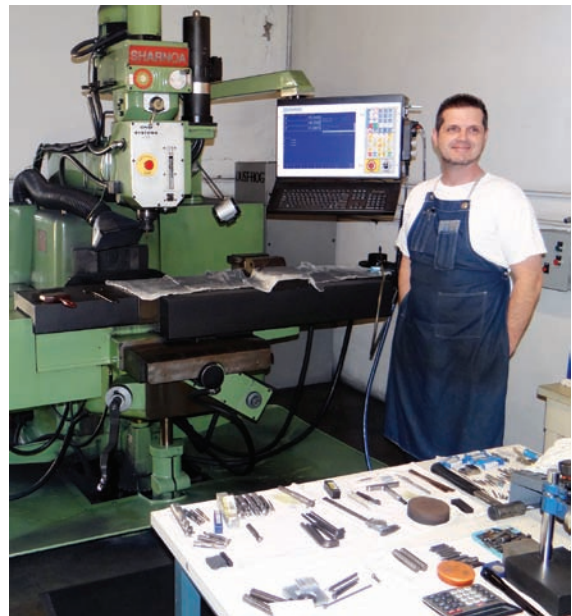
Atticus Overbay, Head of Research and Development, RPM RC Products, with the Sharnoa CNC knee mill with new Centroid M400 CNC control upgrade.
