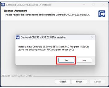
3.) Now select the PLC that is relevant to your machine and Centroid motion control board.
