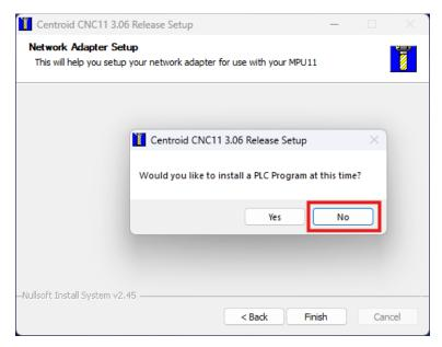
6.) With CNC11 v3.06 now installed, you MUST run and open the CNC11 software at least once, to update the firmware on the Centroid motion controller. When starting CNC11 v3.06 you will see the text in the below image before the CNC11 software starts.
