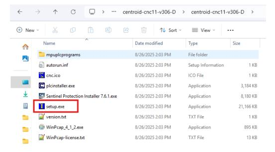
5.) Go through the installer, selecting Mill or Lathe, etc. and when you get to the end, select "No" as to not install a new PLC program.
