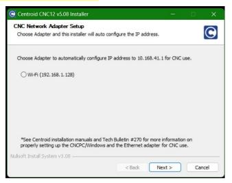
These screens will appear when there is no hardware Ethernet adapter detected by the installer. This means the installer does not "see" the CNC control board Ethernet connection on the CNCPC.
