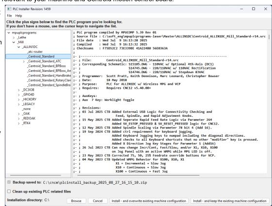
4.) Once you've made your selection for which PLC you want, select "Install – and keep the existing machine configuration."
