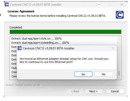
If you don't already have an Ethernet port setup for Centroid CNC use the installer will ask you to choose which one you'd like to configure for CNC use.
