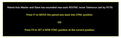
If the controller determines the gantry axis is out of sync by more than .050" the operator is prompted with a message letting him know that the gantry is out of square by more than the P579 value and to press cycle start
