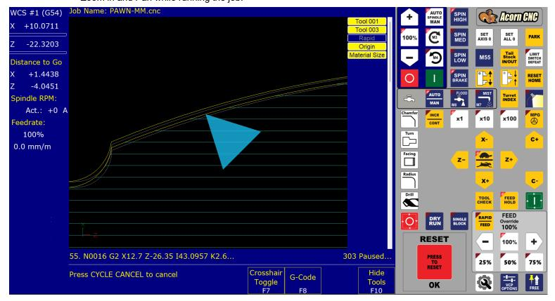
Tool Position is live in the G code backplot so you can see current tool position relative to part program. Jogging in the graphics menu will reflect the cutter position live.
