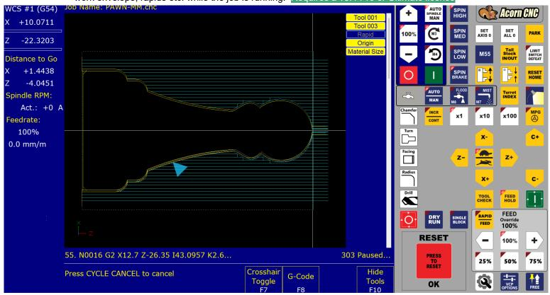
F4 Run, F2 Search → line 54, F10 Accept, cycle start. Rapids set to do not display, Origin set to display (white cross hair), Material Size set to display (dashed line). Zoom in and Pan while running the job.
