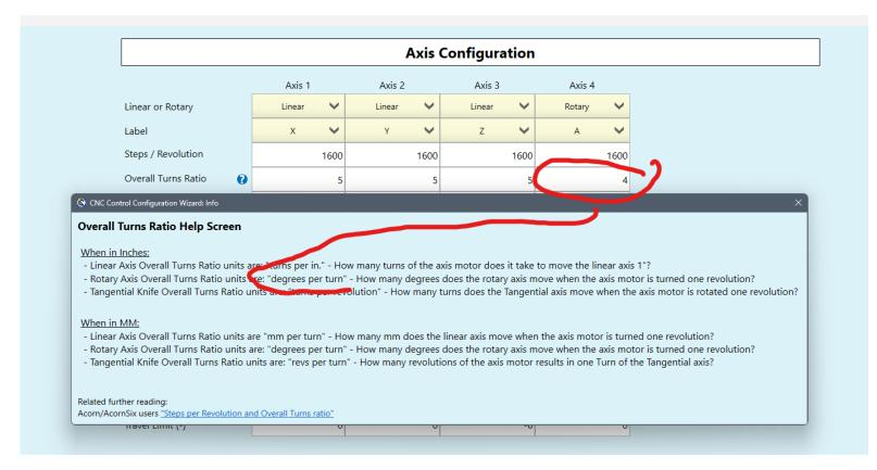
Note: When upgrading from older version of CNC12, DO NOT just type in the old inch number that was in the units of "turns per degree". Please use the new unit of "degrees per turn".
