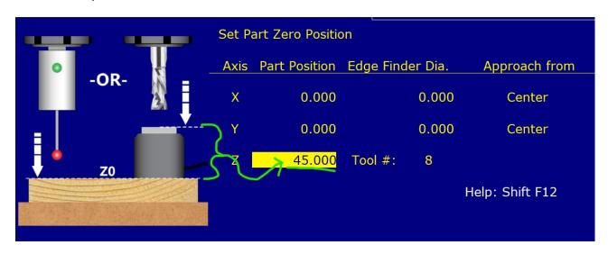
In this example above the TT height is 45 mm, which sets the part zero at the bottom of the TT with "subtract TT height" set to No in the Wizard.
