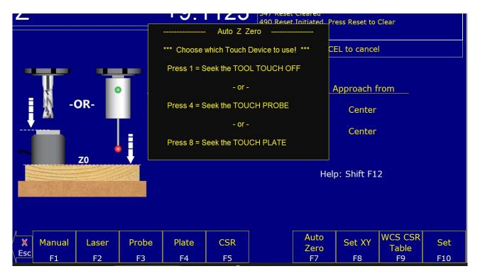
The new Auto Part Z zero macro also employs the new P0 probing cycle command argument which tells the probing cycle to trigger off of any input setup as a probe. So, for instance when probing a TT with a Touch Probe the probing cycle will use whatever input triggers first.
