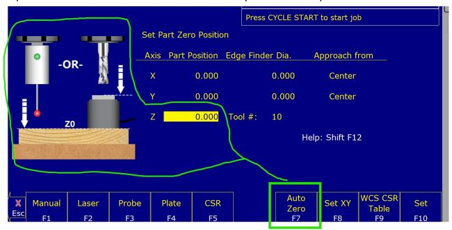
F7 Auto Z zero will now trigger off any type of Probe Input definition. Useful for using a TT to set Part Z zeros. Either the Probe or the TT or Touch Plate can be used with F7 Auto Z zero menu.
