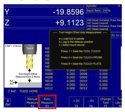
The Auto Tool Height Measurement macro (tool\_offset\_auto\_measure.cnc) will auto recognize all configured touch devices and present the operator with a choice of touch devices to use during the tool height offset measurement cycle.
