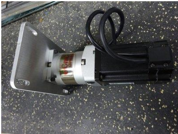
PRS Plate, gearbox & Motor
