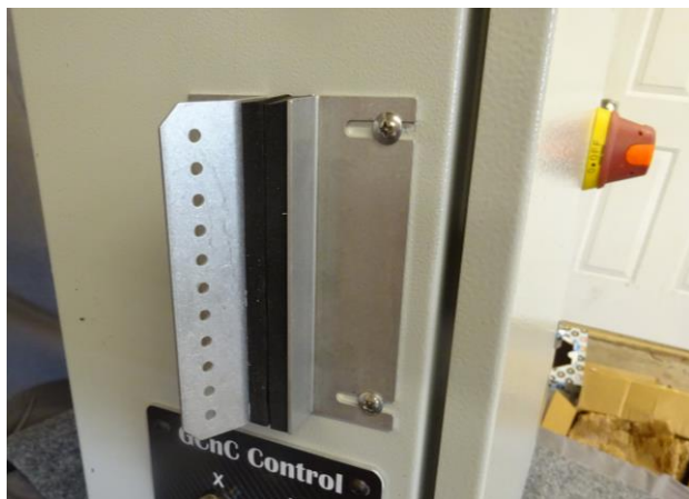
Gasketed Wire Entry with Wire Retainer
