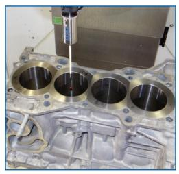
Centroid's DP7 Digitizing Touch Probe. is specifically designed for long stylus operation, which yields ultra precise Block measurements.
